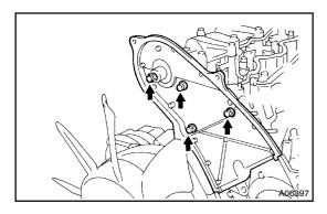
(c) Install the oil seal retainer with the 4 bolts. Uniformly tighten the bolts in several passes.
