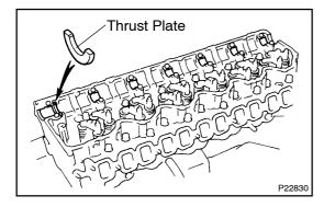
(a) Install the 7 lower camshaft bearings and thrust plate.
