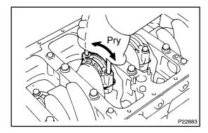
(c) Using the 2 removed connecting rod cap bolts, and remove the connecting cap by wigging the connecting rod cap right and left.
