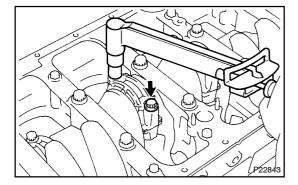
(g) Install the connecting rod cap with the 2 bolts.
