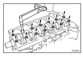
(i) Install the main bearing cap with the 14 bolts (12 pointed head).
