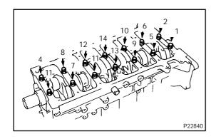
(b) Uniformly loosen and remove the 14 main bearing cap bolts (12 pointed head) in several passes, in the sequence shown.
