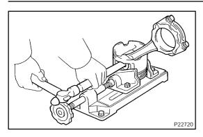
(c) Using a plastic–faced hammer and brass bar, lightly tap out the piston pin and remove the connecting rod.
