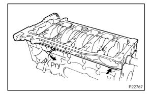
(c) Using a screwdriver, remove the main bearing cap by prying the portions between the main bearing cap and cylinder block.
