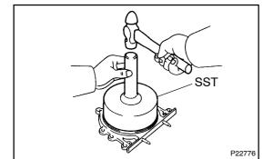
(2) Using SST and a hammer, tap in a new oil seal until its surface is flush with the rear oil seal retainer edge.
