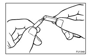
(b) Using a wooden stick, remove the carbon adhering to the nozzle needle tip.
