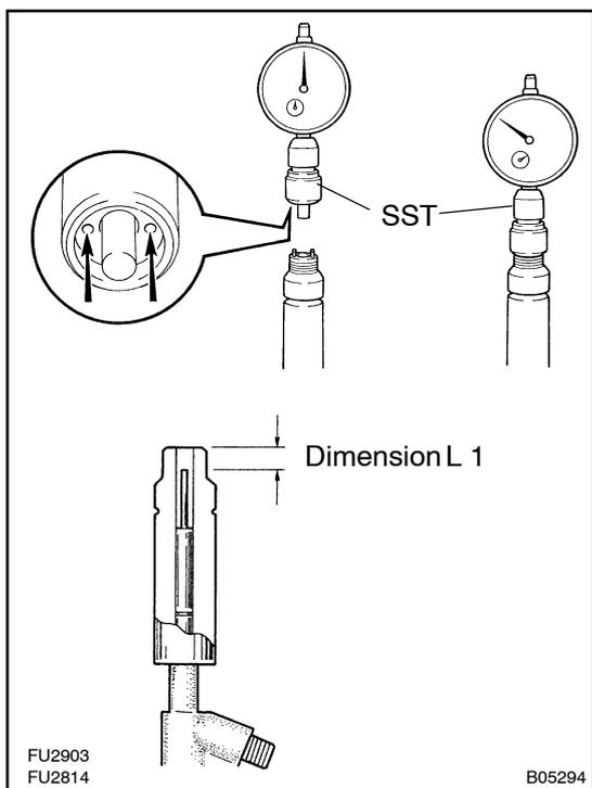
(h) Install SST holes to the straight pins and measure dimension L 1.
