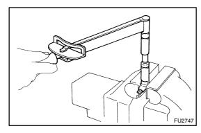
(b) Using a 14 mm deep socket wrench, torque the retaining
