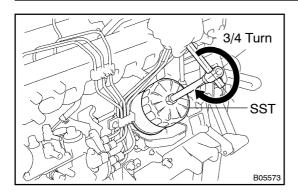
(e) Using SST, give it an additional 3/4 turn to seat the filter. SST 09228–10002
