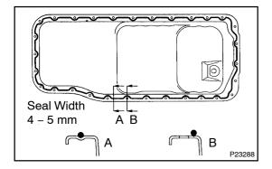
(b) Apply seal packing to the oil pan as shown in the illustration.
