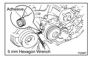
(c) Apply adhesive to 2 or 3 threads of the taper screw plug. **Adhesive:**
