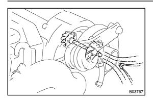
(I) If the engine is running with out the air cleaner, case cover and hose, entry of foreign particles will damage the wheel which run at extremely high speed.
