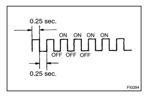
(3) Read the DTC from the check engine warning light (CHK ENG).
