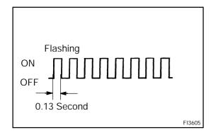
(6) Switch the hand-held tester normal mode to check (test) mode. (Check that the check engine warning light (CHK ENG) flashes.)
