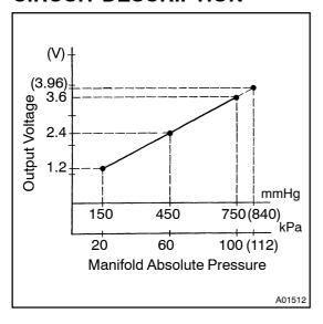
By a built —in sensor unit, the vacuum sensor detects the intake manifold pressure as a voltage. The engine ECU then determines the basic injection duration and basic ignition advance angle based on this voltage.
