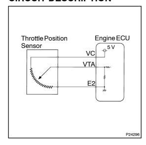
The throttle position sensor is mounted in the throttle body and detects the throttle valve opening angle.
