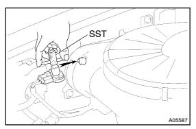
If the CO concentration dose not conform to regulations, adjust by turning the IDLE MIXTURE ADJUSTING SCREW in the variable resister with SST.
