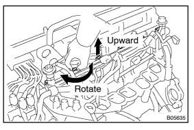
(h) Check that the injectors rotate smoothly. HINT:
