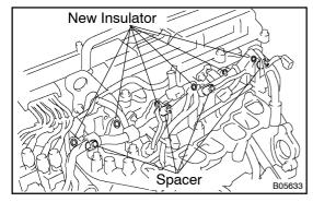
(e) Place 6 new insulators and the 4 spacers in position on the intake manifold.
