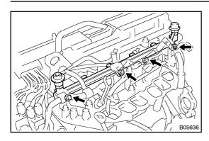
(j) Tighten the 4 bolts holding the delivery pipe to the intake manifold.
