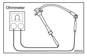
(b) Using an ohmmeter, measure the high —tension cord resistance.
