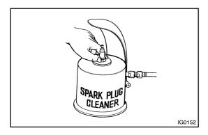
(c) Using a spark plug cleaner or wire brush, clean the spark plug.
