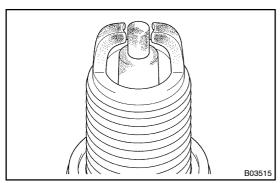
(d) Check the spark plug for electrode wear, thread damage and insulator damage.
