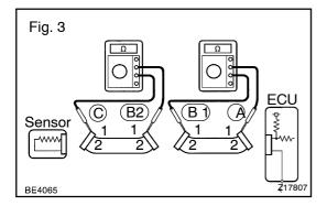
(2) Disconnect connector "B" and measure the resistance between them.
