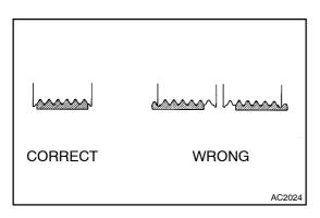
(a) Visually check the drive belt for excessive wear, frayed cords etc.
