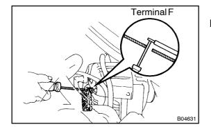
If the voltmeter reading is less than standard voltage, check the IC regulator and alternator as follows:
