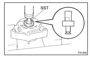
(b) Using SST and a press, press out the bearing. SST 09950-60010 (09951-00260, 09952-06010)
