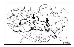
(f) Install the water inlet and housing assembly with the 2 bolts. Alternately tighten the bolts.
