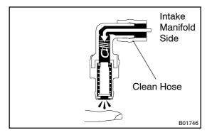
(b) Blow air into the intake manifold side, and check that air passes through with difficulty.
