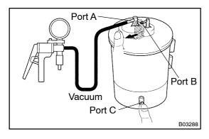
(b) Apply vacuum ( 1.96 kPa (20 gf/cm , 0.28 psi)) to port A, check that the vacuum does not decrease when port B and C are closed, and check that the vacuum decreases when port B is released.
