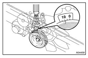
(b) Using a timing light, check the ignition timing. **Ignition timing:**
