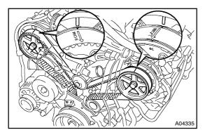
(b) Check that the timing marks of the camshaft timing pulleys and timing belt rear plates aligned.
