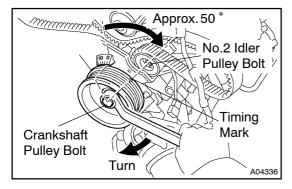
(c) Turn the crankshaft pulley approx. 50 ° clockwise, and put the timing mark of the crankshaft pulley in line with the centers of the crankshaft pulley bolt and the idler pulley bolt.
