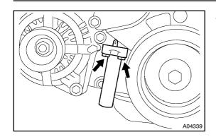
Alternately loosen the 2 bolts, and remove them, the belt tensioner and dust boot.
