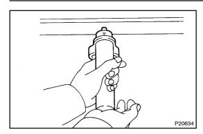
(b) Hold the tensioner with both hands and push the push rod strongly as shown to check that it doesn't move.
