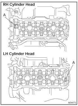
S Do not drop the plate washer for cylinder head bolt into portion A of the cylinder head. If dropped into portion A, the plate washer will pass through the cylinder head and cylinder block into the oil pan.
