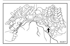
(b) Lift the cylinder head from the dowels on the cylinder block, and place the 2 cylinder heads on wooden blocks on a bench.
