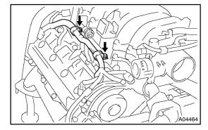
(f) Disconnect the 2 wire clamps from the wire clamp bracket on the RH delivery pipe.
