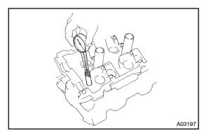
(c) Using a caliper gauge, measure the bushing bore diameter of the cylinder head.
