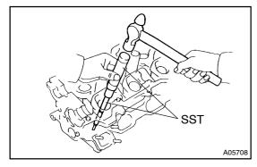
(b) Using SST and a hammer, tap out the guide bushing. SST 0920 1–01055,
