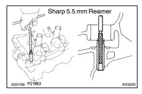
(g) Using a sharp 5.5 mm reamer, ream the guide bushing to obtain the standard specified clearance (See page EM-41) between the guide bushing and valve stem.
