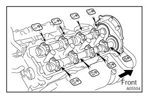
(6) Install the front bearing cap.
