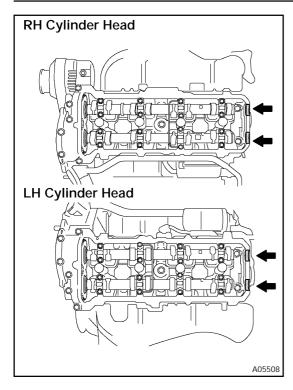
(c) Install the 4 semi-circular plugs to the cylinder heads.
