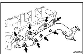
(b) Install the exhaust manifold with 8 new nuts. Uniformly tighten the nuts in several passes.
