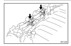
(k) Connect the 2 wire clamp to the wire clamp bracket on the RH delivery pipe.
