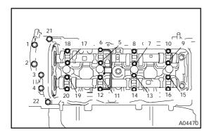
(11) Uniformly tighten the 22 bearing cap bolts in several passes, in the sequence shown.
