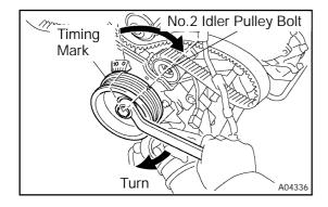
(a) Set the crankshaft pulley position. Turn the crankshaft pulley clockwise or counterclockwise, and put the timing mark of the crankshaft pulley in line with the centers of the crankshaft pulley bolt and idler pulley bolt.
