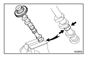
(c) Mount the hexagon wrench head portion of the camshaft in a vise.
