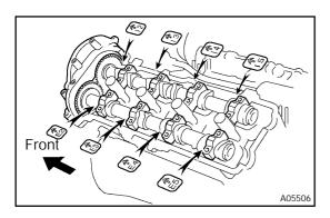
(6) Install the front bearing cap.
