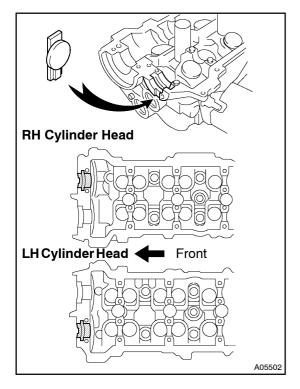
(c) Install the 2 camshaft housing plugs to the cylinder heads.
