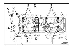
(9) Apply a light coat of engine oil on the threads and under the heads (D and E) of the bearing cap bolts.
