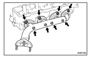
(b) Install the exhaust manifold with 8 new nuts. Uniformly tighten the nuts in several passes.
