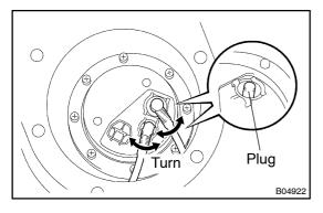
(c) Pull out the fuel main tube and return tube.
