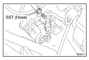
(c) Connect SST (hose) and fuel tube connector to the fuel filter outlet.
