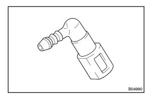
(b) Purchase the new fuel main hose and take out the fuel tube connector from its hose.
