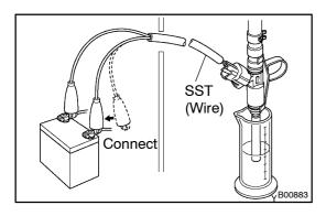
(q) Connect SST (wire) to the injector and battery for 15 seconds, and measure the injection volume with a graduated cylinder. Test each injector 2 or 3 times.
