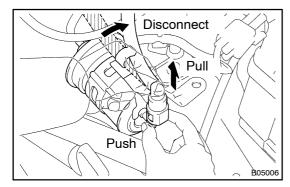
(a) Disconnect the fuel inlet hose (fuel tube connector) from the fuel filter.
