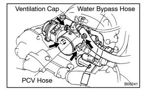
(b) Install a new gasket and the throttle body with the 2 bolts and 2 nuts.
