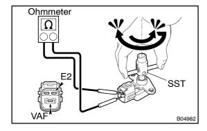
(c) Using SST, turn the idle mixture adjusting screw fully counterclockwise.
