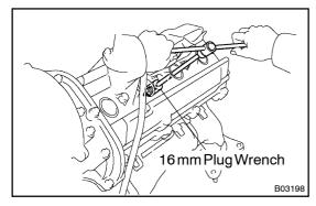
(c) Using a 16 mm plug wrench, remove the spark plugs.
