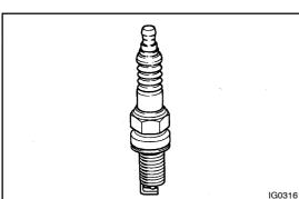
(d) Check the spark plug for thread damage and insulator damage.
