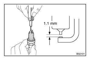
(e) Check the spark plug electrode gap.
