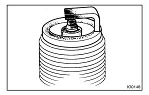
(d) Check the spark plug for thread damage and insulator damage.
