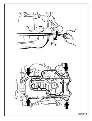
(b) Using a screwdriver, remove the No. 1 oil pan by plying between the oil pan and cylinder block in the sequence shown.
