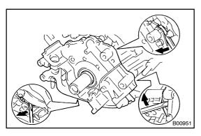
(b) Using a screwdriver, remove the oil pump by plying the portions between the oil pump and cylinder block.
