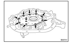
(b) Install the pump body cover with the 10 screws.
