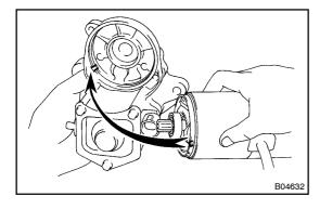
(c) Pull out the field frame together with the armature from the magnetic switch assembly.
