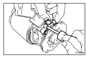
Check that the positive (+) lead wires are not grounded.
