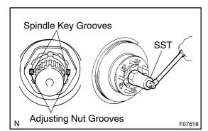
(e) Tighten the adjusting nut in the tightening direction so that the grooves of the adjusting nut are aligned with on the key grooves before and after spindle.
