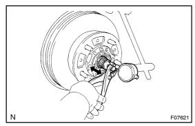
(e) Using a dial indicator, check the backlash near the center of the axle shaft, while pulling the bolt with pliers.
