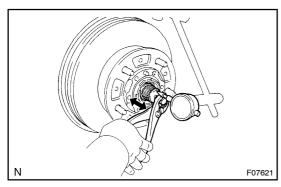
(e) Using a dial indicator, check the backlash near the center of the drive shaft, while pulling the bolt with pliers.
