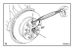
(f) Using a spring tension gauge, measure the preload. **Preload (at starting):**
