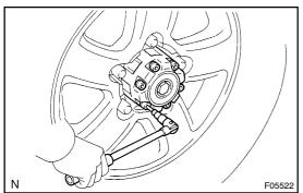
(c) Using a 8 mm hexagon wrench, install the 6 hexagon bolts.
