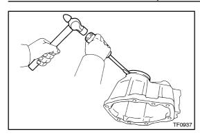
(b) Using a screwdriver and hammer, tap the dust deflector from the front extension housing and remove it.
