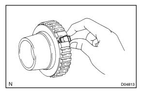
(c) Remove the 3 No. 1 synchromesh shifting keys and springs from the drive clutch hub.
