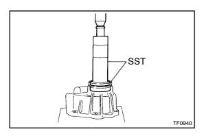
(b) Using SST and a press, remove the ball bearing. SST 093 16–60011 (09316–00011, 093 16–00071)
