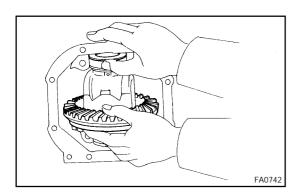
(e) Select a ring gear teeth side plate washer so that is no clearance between the outer race and case.
