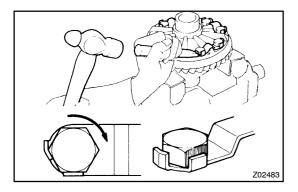
(g) Using a chisel and hammer, stake the 5 lock plates. HINT:
