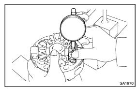
(e) Using a dial indicator, holding the side gear and spider, measure the side gear backlash,
