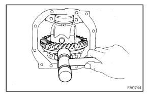
(b) Tap on the ring gear with a plastic hammer so that the washer fits to the bearing.
