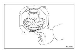
(d) Select a plate washer for back side ring gear, using the backlash as reference.
