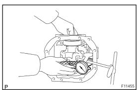
(c) Using a dial indicator, measure the side gear backlash while holding one pinion gear toward the differential case.
