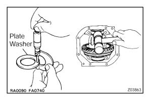
(b) Using the backlash as a reference, install a new washer of 0.06 – 0.09 mm (0.0024 – 0.0035 in.) thicker than the washer removed.
