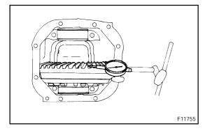
(j) Using a dial indicator, measure the ring gear backlash. Backlash: 0.13 – 0.18 mm (0.0051 – 0.0070 in.)
