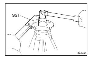
(d) Using SST to hold the flange and adjust the drive pinion preload by tightening the nut.
