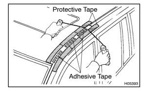
(g) Cut the adhesive tape by pulling the piano wire as shown.
