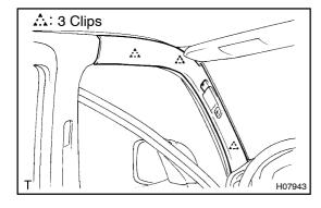
(c) Using a screwdriver, remove the front pillar garnish.
