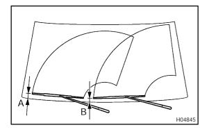
(c) Adjust the installation positions of the wiper arms to the positions as shown in the illustration.
