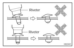
S Loose tightening may result from either tilting the riveter while handling or the riveter not connecting to the material.
