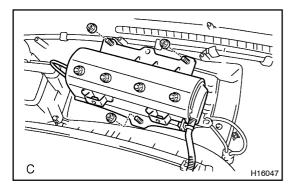
(b) Remove the 3 nuts and front passenger airbag assembly.
