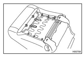
(c) Remove the 10 hog rings and 2 clamps.
