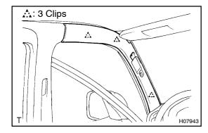
(c) Using a screwdriver, remove the front pillar garnish. HINT:
