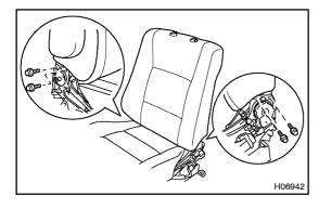
(b) Remove the 4 bolts and seatback assembly.
