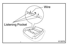
(b) Thread the wire through the listing pocket after setting the seat heater to the seat cushion cover.
