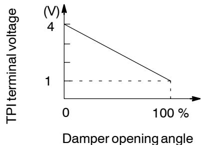
This sensor detects the position of the air inlet damper and sends the appropriate signals to the A/C amplifier.
