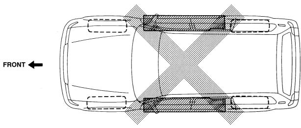
NOTICE: Never use the plate type lift —using it to lift up the vehicle will cause the body shape to warp.
