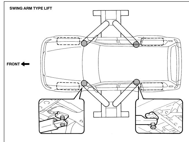
NOTICE: When lifting the vehicle, place the supports correctly at the positions shown above.
