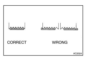
(a) Visually check the drive belt for excessive wear, frayed cords etc.
